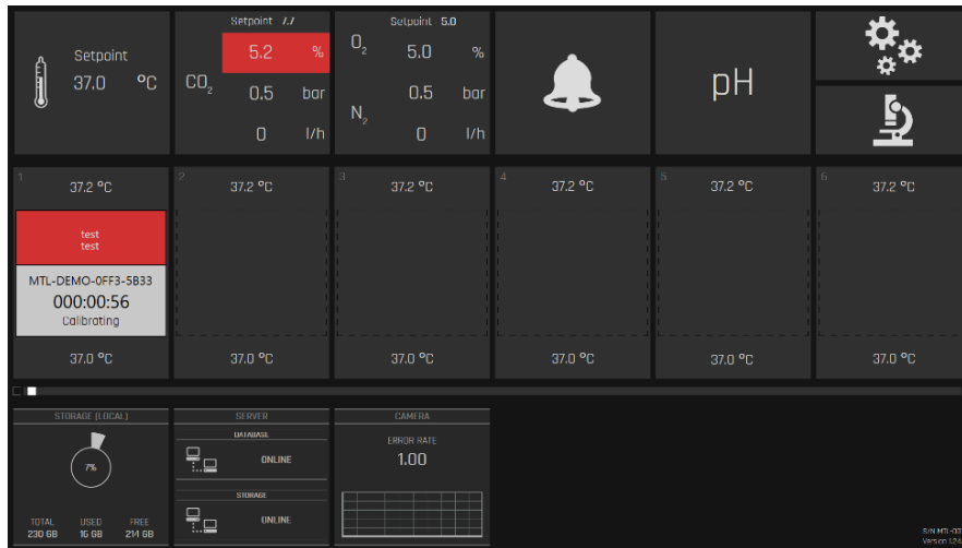
Figure 20.38 CO 2 concentration alarm view
